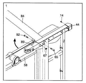
With the help of a second person, carefully tip the treadmill onto its right side. Do not fully fold the treadmill until it is completely assembled.
