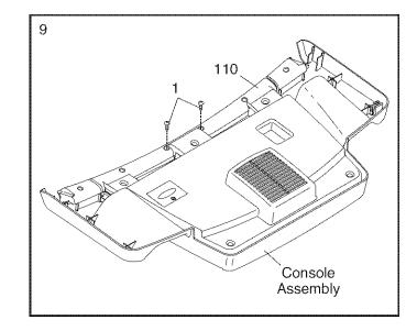
Set the Pulse Bar (110) on the Left and Right Uprights (77, 92). Attach the Pulse Bar with four #10 x 3/4" Screws (4) and four #10 Star Washers (12). Start all four Screws before firmly tightening any of them. Be careful not to pinch the Wire Harness (91).
