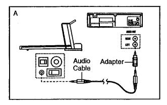
B. Plug one end of the audio cable into the jack on the front of the treadmill near the power cord. Plug the other end of the cable into the included adapter. Plug the adapter into an RCA Y-adapter (available at electronics stores). Next, remove the wire that is currently plugged into the AUDIO OUT jack on your VCR and plug the wire into the unused side of the Y-adapter. Plug the Y-adapter into the AUDIO OUT jack on your VCR.
