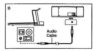
C. Plug one end of the audio cable into the jack on the front of the treadmill near the power cord. Plug the other end of the cable into a 3.5mm Y-adapter (available at electronics stores). Plug the Y-adapter into the PHONES jack on your stereo. Plug your headphones into the other side of the Y-adapter.
