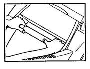
tacts—avoid moving your hands. When your pulse is detected, the heart-shaped indicator in the Calories/Fat Calories/Heart Rate display will flash, and then your heart rate will be shown. For the most accurate heart rate reading, continue to hold the contacts for about 15 seconds.
