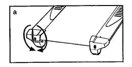
b. If the walking belt slips when walked on, first remove the key and UNPLUG THE POWER CORD. Using the allen wrench, turn both rear roller bolts clockwise, 1/4 of a turn. When the walking belt is correctly tightened, you should be able to lift each side of the walking belt 3 to 4 inches off the walking platform. Be careful to keep the walking belt centered. Plug in the power cord, insert the key and carefully walk on the
