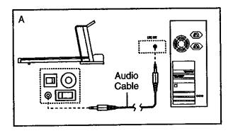
B. Plug one end of the audio cable into the jack on the front of the treadmill near the power cord. Plug the other end of the cable into a 3.5mm Y-adapter (available at electronics stores). Plug the Y-adapter into the PHONES jack on your computer. Plug your headphones or speakers into the other side of the Y-adapter.
