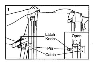
2. Hold the treadmill firmly with both hands, and lower the treadmill to the floor. Do not drop the treadmill frame to the floor. CAUTION: To decrease the possibility of injury, bend your legs and keep your back straight.
