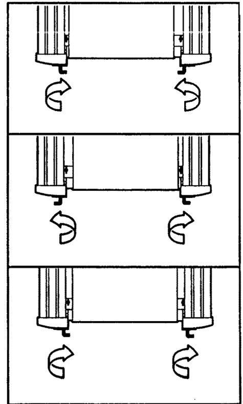
To convert the CROSS WALK to the stowaway position, first unplug the power cord. Remove the lock knob and washer from the upright and lay the upright on the walking belt. Keep the lock knob and washer in a secure location.
