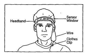
IMPORTANT: To avoid static build-up that may damage the console, wear the pulse sensor only while you are on the treadmill.
