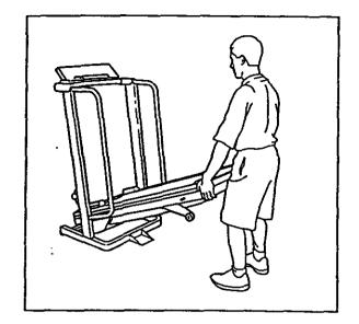
Move your right hand to the position shown at the right, and hold the treadmill firmly. Using your left hand, lift the storage latch. Raise the treadmill until the locking pin snaps into the storage latch. Make sure that the locking pin is inside the storage latch, and that the storage latch is fully closed.
