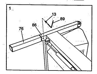
Attach six Base Pads (43) to the Base (86) and the Base Extensions (76) in the indicated locations. Note: One extra Base Pad may be included.
