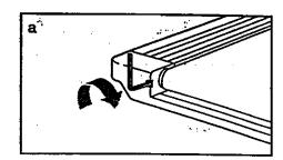
b. If the walking belt has shifted to the right, first remove the key and UNPLUG THE POWER CORD. Using the allen wrench, turn the left rear roller adjustment bolt counterclockwise 1/4 of a turn. Plug in the power cord, insert the key and run the treadmill for a few minutes. Repeat until the walking belt is centered.
