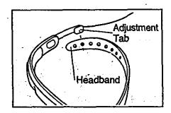
cise, the headband may expand slightly during the first few minutes of use. It may be necessary to readjust the headband periodically.
