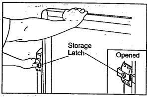
Hold the treadmill firmly with both hands, and lower the treadmill to the floor. Caution: To avoid pinching your hands, do not hold the treadmill in the locations indicated by the arrows. To decrease the possibility of injury, bend your legs and keep your back straight.
