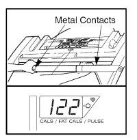
avoid moving your hands. When your heart rate is detected, the heart-shaped indicator in the CALS/FAT CALS/PULSE display will flash steadily and a "P" will appear. After a few seconds, your heart rate will be shown. For the most accurate heart rate reading, continue to hold the contacts for about 15 seconds.
