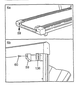
7. Make sure that all parts are tightened before you use the treadmill. Keep the included allen wrench in a secure place. The allen wrench is used to adjust the walking belt (see page 20). To protect the floor or carpet from damage, place a mat under the treadmill.
