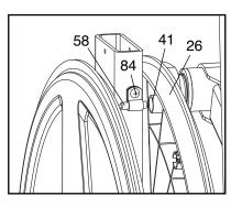
(84). Slide the Reed Switch slightly closer to or away from the Magnet, and then retighten the Screw. Rock the Left Pedal Disc forward and backward just enough that the Magnet passes the Reed Switch repeatedly. Repeat until the console displays correct feedback. When the Reed Switch is correctly adjusted, reattach the shields. Note: If you have questions as to which screw should be in which hole, see EXPLODED DRAWING B on page 27 and the PART LIST on page 24.
