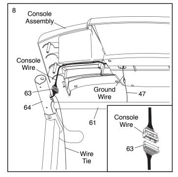
9. Insert the wires into the Right Handrail (64) through the indicated hole as you set the console assembly on the Left and Right Handrails (59, 64). **Make sure that no wires are pinched.**
