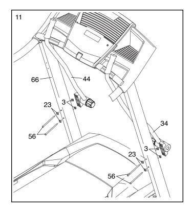
Orient the Latch Pin Assembly (68) so that the knob is on the indicated side. Attach the Latch Pin Assembly with the Latch Spacer (82) to the Left Upright (66) with two #10 x 1 1/2" Screws (8). Start both Screws, and then tighten them. Be careful not to overtighten the Screws.
