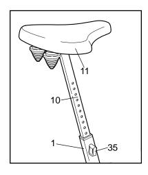
Pin (35). Align one of the holes in the Seat Post (10) with the hole in the Frame (1). Insert the Seat Pin into the Frame and the Seat Post. Caution: Make sure to insert the Seat Pin through one of the holes in the Seat Post; do not insert the Seat Pin under the Seat Post.
