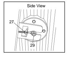
(27) clockwise; to loosen the Belt, turn the Adjustment Nuts counterclockwise. Make sure that the Flywheel is straight and tighten the Axle Nuts (29). Reattach the side shields.
