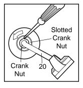
slotted crank nut is properly tightened, retighten the crank nut.
