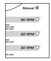
programs will be selected in the following order: the manual mode, the 6 MPH/30 RPM program, the 12 MPH/60 RPM program, and the 18 MPH/ 90 RPM program. Note: Once you select a pacer program, you can reselect the manual mode by repeatedly pressing the program button.
