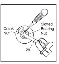
in one of the slots in the slotted bearing nut. Lightly tap the screwdriver with a hammer to turn the slotted bearing nut counterclockwise until the arms are no longer loose. **Do not overtighten the slotted bearing nut.** When the slotted bearing nut is properly tightened, tighten the crank nut.
