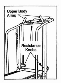
To vary the intensity of your upper body exercise, the resistance of the upper body arms can be adjusted. To increase the resistance, turn the resistance knobs clockwise; to decrease the resistance, turn the knobs counterclockwise.
