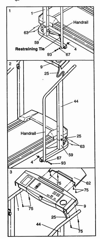
4. With the help of a second person, carefully lower the Left and Right Uprights (1, 44) until the handrails are resting on the floor.
