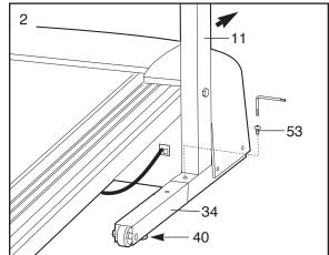
3. Hold one of the Handrails (1) at an angle as shown and insert the upper end as far as possible into the right Upright (11). Keep the lower end of the Handrail away from the treadmill to avoid scratching the finish. Next, rotate the lower end of the Handrail to the position shown by the dotted line.
