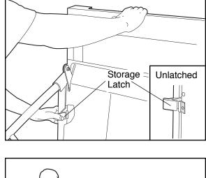
2. Hold the treadmill firmly with both hands, and lower the treadmill to the floor. To decrease the possibility of injury, bend your legs and keep your back straight.
