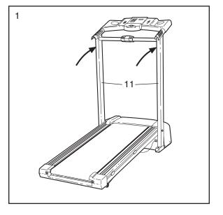
Insert one of the Extension Legs (34) into the treadmill as shown. (Note: It may be helpful to tip the Uprights [11] in the direction shown by the arrow as you insert the Extension Leg.) Make sure that the Base Pad (40) is on the indicated side of the Extension Leg. Attach the Extension Leg with an Extension Leg Screw (53). Be sure to push on the head of the Extension Leg Screw while tightening it.
