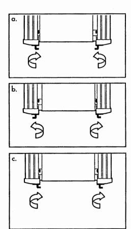
Before converting the CROSS WALK to the stowaway position, turn the resistance control (see the drawing on page 8) counterclockwise until the control turns freely. Next, unplug the power cord. Remove the lock knob and washer from the upright and lay the upright and the upper body arms on the walking belt. Keep the lock knob and washer in a secure location.
