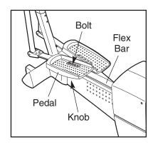
upward, slide the pedal forward or backward to the desired position, and then retighten the knob. Make sure that both pedals are in the same position.
