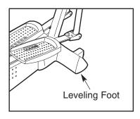
under the front stabilizer until the rocking motion is eliminated.
