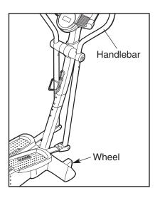
to the desired location. Then, place one foot against one of the wheels and lower the elliptical crosstrainer. Due to the size and weight of the elliptical crosstrainer, use extreme caution while moving and lowering it.
