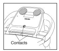
To measure your heart rate, **stand on the foot rails** and hold the pulse bar with your palms on the metal contacts for approximately ten seconds; **avoid moving your hands.** When your pulse is detected, a heart symbol in the lower right display
