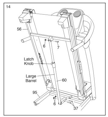
15. Make sure that all parts are properly tightened before you use the treadmill. If there are sheets of plastic on the treadmill decals, remove the plastic. To protect the floor or carpet, place a mat under the treadmill. Keep the included hex keys in a secure place; one of the hex keys is used to adjust the walking belt (see pages 26 and 27).
