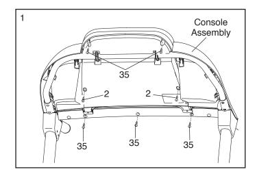
Carefully lift the console assembly off of the Console Base (103). Locate the Pulse Wire (A) on the console assembly.
