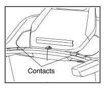
To measure your heart rate, stand on the foot rails and place your hands on the metal contacts—avoid moving your hands. When your pulse is detected, your heart rate will be shown. For the most accurate heart rate reading, continue to hold the contacts for about 15 seconds.
