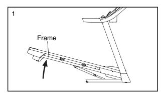
Raise the frame until the storage latch locks in the storage position. CAUTION: Make sure that the storage latch locks.
