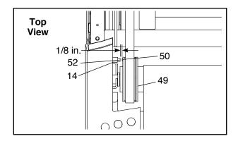
Next, locate the Reed Switch (52) and the Magnet (50) on the left side of the Pulley (49). Turn the Pulley until the Magnet is aligned with the Reed Switch. Make sure that the gap between the Magnet and the Reed Switch is about 1/8 in. (3 mm). If necessary, loosen the #8 x 3/4" Truss Head Screw (14), move the Reed Switch slightly, and then retighten the Screw. Reattach the Motor Hood (not shown), and run the treadmill for a few minutes to check for a correct speed reading.
