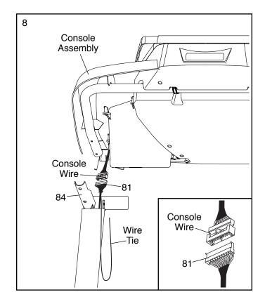
Set the console assembly on the Handrails (84).
