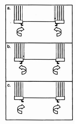
correct, you should be able to lift each side of the walking belt 3-4 inches off the walking platform. The center of the walking belt should just touch the surface of the walking platform. Be careful to keep the walking belt centered on the walking platform.
