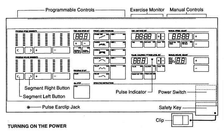
Make sure that the safety key is removed from the console. Plug the power cord in. (See PLUGGING IN THE POWER CORD on page 5.)
