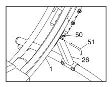
the Incline Pin into the Front Leg (26) and into one of the three adjustment holes in the Incline Leg (50).
