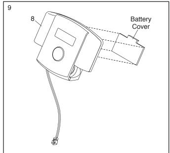
10. Remove the three M3 x 15mm Screws (24) from the Console (8), and remove the back of the Console.
