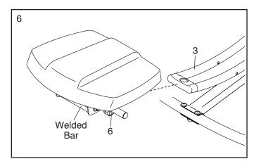
7. Move the Carriage (6) to the position shown, and align the indicated hole in the Carriage with the corresponding hole (not shown) in the Pivot Frame (3).
