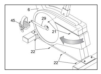
Remove the four M4 x 16mm Screws (22) and the two M4 x 32mm Screws (21) from the Left Side Shield (6). Grasp both Side Shields at the top and gently pull them apart. Make sure that the arm of the Crank (29) is in the position shown in the drawing above. Hold the Left Side Shield at the rear and pull it gently away from the frame. Work the Left Side Shield forward off the arm of the Crank and remove it.
