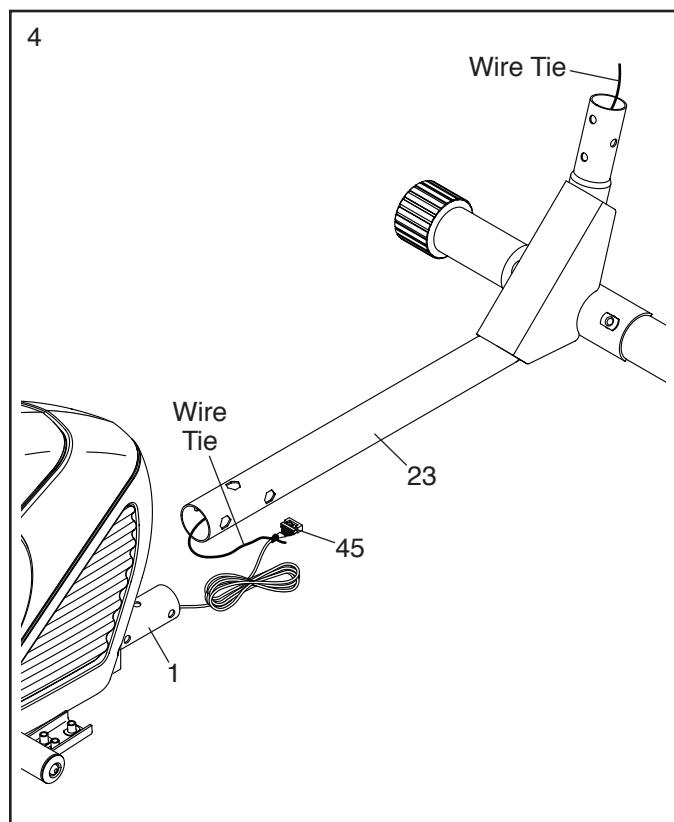
5. **Tip: Avoid pinching the Main Wire Harness (45).** Slide the Front Frame (23) onto the Rear Frame (1). Attach the Front Frame with three M10 x 60mm Bolts (61) and three M10 Locknuts (48); **make sure that the Locknuts are in the hexagonal holes. Do not tighten the Bolts yet.**
