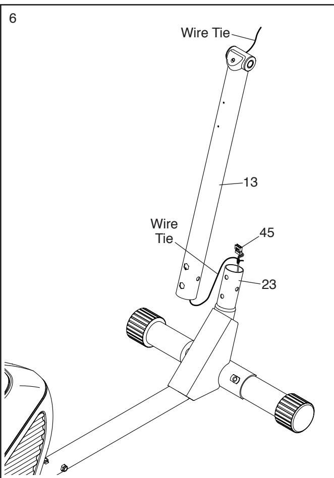
7. **Tip: Avoid pinching the Main Wire Harness (45).** Slide the Upright (13) onto the Front Frame (23). Attach the Upright with three M10 x 60mm Bolts (61) and three M10 Locknuts (48); **make sure that the Locknuts are in the hexagonal holes. Do not fully tighten the Bolts yet.**
