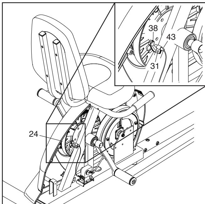
Next, rotate the Pulley (24) until a Magnet (38) is aligned with the Reed Switch (43). Slide the Reed Switch slightly toward or away from the Magnet. Then, retighten the M4 x 12mm Screw (31).
