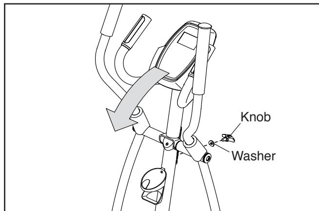
Next, lift a pedal, pivot the brace downward, and insert the end of the brace into the pedal carriage. **Make sure that the brace is securely inserted into the pedal carriage. Repeat this action for the other pedal.**
