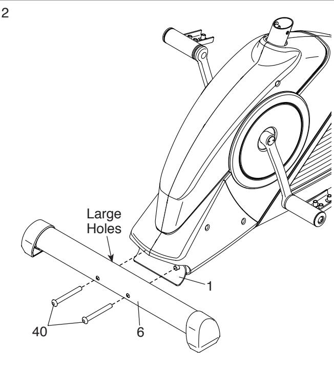
3. Orient the Front Stabilizer (2) so that the large holes are facing the Front Frame (23). Attach the Front Stabilizer to the Front Frame with two M10 x 65mm Screws (40).
