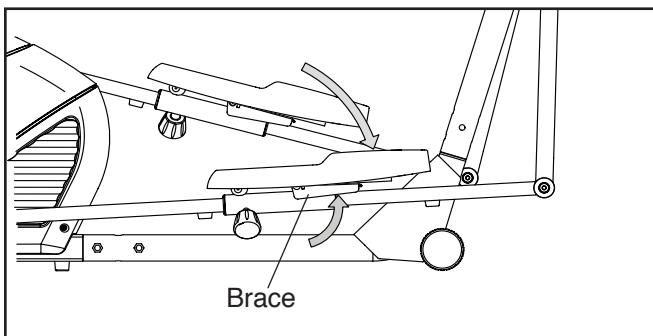
To mount the hybrid trainer in the elliptical mode, hold the handlebars or the upper body arms and step onto the pedal that is in the lower position. Then, step onto the other pedal.
