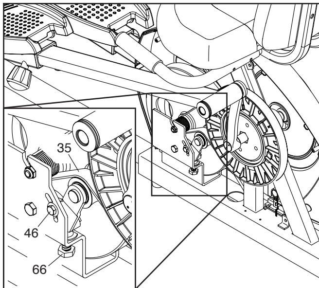
When the Drive Belt (35) is tight, tighten the M6 x 20mm Hex Screw (46). Then, reattach the shields.
