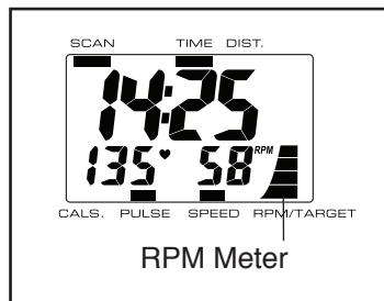
To cancel the scan mode, press the Display button. The indicator below the word SCAN will disappear. The upper section of the display will then show only the elapsed time. If you press the Display button again, the upper section of the display will show only the distance pedaled. To select the scan mode again, press the Display button repeatedly until an indicator appears below the word SCAN.
