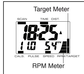
As the target meter changes in height during the workout, adjust your pedaling speed so that the same number of bars appears in both meters. If your pedaling speed is slower than the current target speed, an arrow will appear next to the RPM meter to prompt you to increase your speed; if your pedaling speed is faster than the target speed, an arrow will prompt you to decrease your speed.
