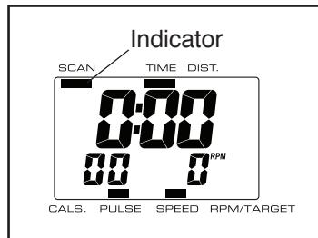
As you exercise, the upper section of the display will alternately show the elapsed time and the distance that you have pedaled; the lower left section of the display will show the number of calories you have burned. The lower right section of the display will show your pedaling speed.
