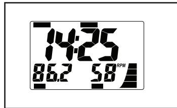
In addition, the RPM meter on the right side of the display will provide a visual representation of your pedaling speed. As you increase or decrease your pace, bars will appear or disappear in the RPM meter.
