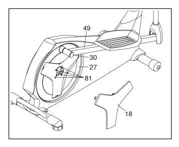
Next, remove the M8 x 12mm Screws (81) from the Right Pedal Disc (27),
