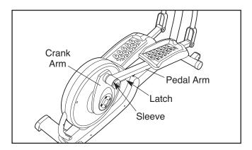
Next, raise the pedal arms until they touch the magnets on the upper body arms; the magnets will hold the pedal arms in place. Then, hold the handle and lift the frame until it locks in a vertical position.
