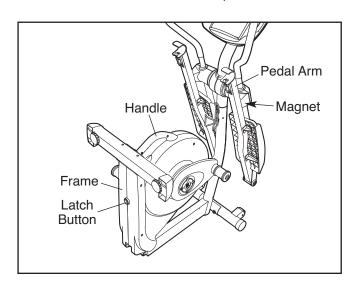
To use the elliptical, first hold the handle, press the latch button, and lower the frame.
