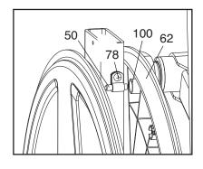
Reed Switch slightly closer to or away from the Magnet, and then retighten the Screw. Rock the Pulley Disc forward and backward just enough that the Magnet passes the Reed Switch repeatedly. Adjust the Screw until the console displays correct feedback. When the Reed Switch is correctly adjusted, reattach the shields. Note: If you have questions as to which screw should be in which hole, see EXPLODED DRAWING B on page 27 and the PART LIST on page 24.
