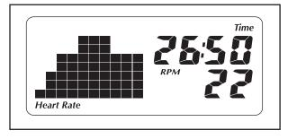
During both workouts, the console will regularly compare your heart rate to the target heart rate setting for the current segment of the workout. If your heart rate is too far below or above the target heart rate setting, the resistance of the pedals will automatically increase or decrease to bring your heart rate closer to the target heart rate setting. Each time the resistance changes, the resistance level will appear in the display for a few seconds to alert you.
