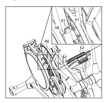
Next, loosen, but do not remove, the two indicated M4 x 16mm Screws (61). Slide the Reed Switch (58) slightly toward or away from the Magnet (41). Then, retighten the M4 x 16mm Screws.
