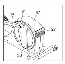
Remove the four M4 x 16mm Screws (not shown) from the Large Storage Foot (27), and then remove the Large Storage Foot. Remove the two M4 x 16mm Screws (not shown) from the Top Shield (37), and then use a flat screwdriver to pry the Top Shield upward off the elliptical. Then, pry the left Pedal Disc (36) off the elliptical.
