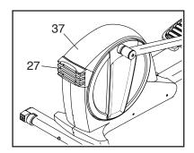
M4 x 16mm Screws (not shown) from the Top Shield (37), and then use a flat screwdriver to pry the Top Shield upward off the elliptical.
