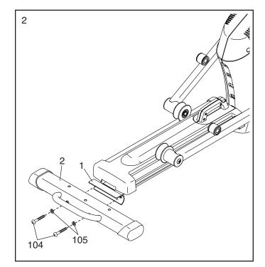
Press the Cover Mounts (106) on the underside of the Rear Stabilizer Cover (15) into the Rear Stabilizer (2).
