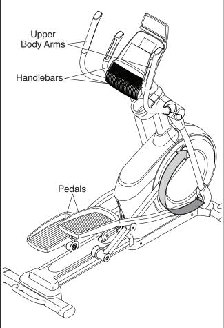
To dismount the elliptical, wait until the pedals come to a complete stop. **Note: The elliptical does not have a free wheel; the pedals will continue to move until the flywheel stops.** When the pedals are stationary, step off the higher pedal first. Then, step off the lower pedal.
