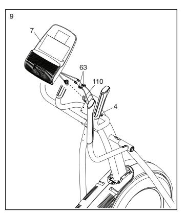
10. **Tip: Avoid pinching the wires.** Attach the Console (7) to the Upright (4) with four M4 x 16mm Screws (101); **start all of the Screws, and then tighten them.**
