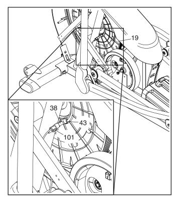
Loosen, but do not remove, the indicated M4 x 16mm Screw (101). Slide the Reed Switch (38) slightly closer to or away from the Magnet (43), and then retighten the Screw.
