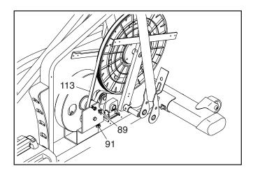
Reattach the right shield, the right roller arm, the right pedal arm, the shield cover cap, and the shield cover. Then, plug in the power adapter.
