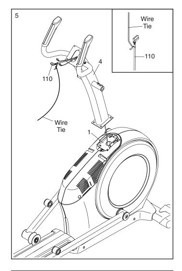
6. **Tip: Avoid pinching the Main Wire (110). Avoid damaging the indicated plastic tabs.**Have a second person hold the Upright (4) on the Frame (1).
