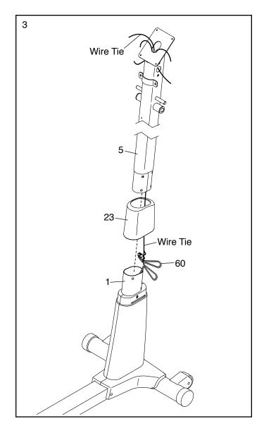
4. **Tip: Avoid pinching the Wire Harness (60).** Insert the Upright (5) into the Frame (1).
