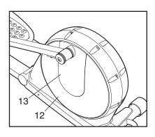
using a flat screwdriver. Next, remove the four screws (not shown) from the center of the left Disc (12). Gently rotate the Disc Cover and the Disc away from the elliptical exerciser.
