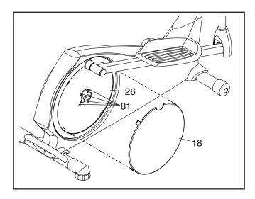
Then, remove the M8 x 12mm Screws (81) from the right Pedal Disc (26), and gently rotate the right Pedal Disc out of the way.
