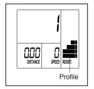
When you select a preset workout, the duration of the workout will appear in the upper display and a profile of the resistance levels of the workout will scroll across the center display.
