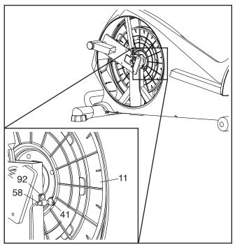
Next, rotate the Pulley (11) until a Magnet (41) is aligned with the Reed Switch (58). Slide the Reed Switch slightly toward or away from the Magnet. Then, retighten the M4 x 16mm Screw (92).
