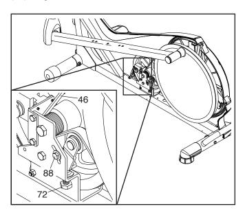
When the Drive Belt (46) is tight, tighten the Pivot Screw (88).
