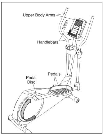
Push the pedals until they begin to move with a continuous motion. Note: The pedal discs can turn in either direction. It is recommended that you move the pedal discs in the direction shown by the arrow; however, for variety, you can turn the pedal discs in the opposite direction.
