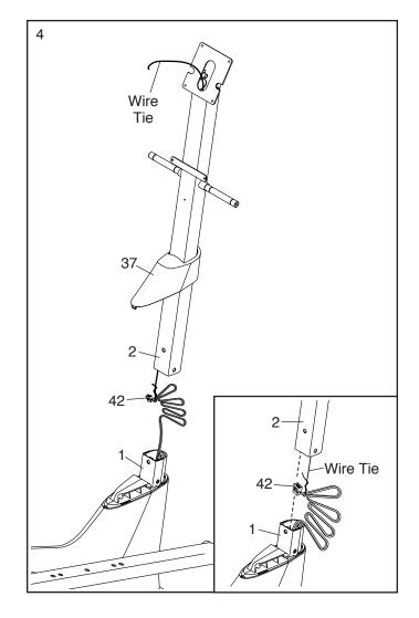
5. Slide the Upright (2) onto the Frame (1). Tip: Have a second person hold the Top Shield Cover (37) out of the way.
