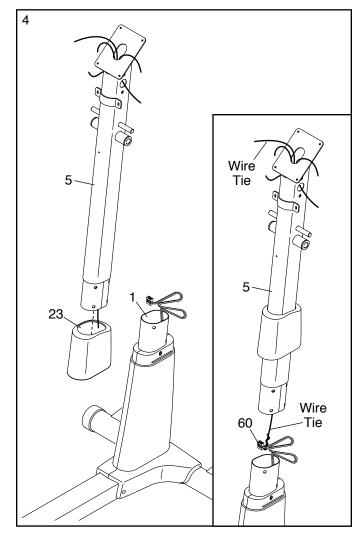
5. **Tip: Avoid pinching the Wire Harness (60).** Insert the Upright (5) into the Frame (1).
