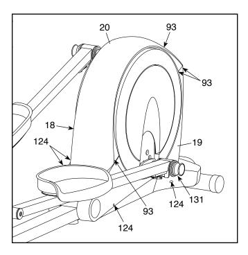
Next, remove the M4 x 16mm Screws (93), the M4 x 42mm Screws (124), and the M4 x 25mm Screw (131) from the Right and Left Shields (18, 19). **Make sure to note which size of Screw you remove from each hole.** Then, gently remove the Left Shield.
