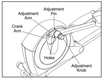
Pivot the adjustment arm back and forth slightly to make sure that the adjustment pin is engaged in one of the holes in the crank arm.
