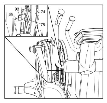
Next, rotate the Large Pulley (74) until a Magnet (75) is aligned with the Reed Switch (69). Slide the Reed Switch slightly toward or away from the Magnet. Then, retighten the M4 x 16mm Screw (93).
