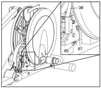
When the Drive Belt (38) is tight, tighten the Pivot Screw (97).
