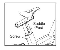
saddle post, loosen the adjustment screw, move the saddle post upward or downward, and then retighten the adjustment screw.
