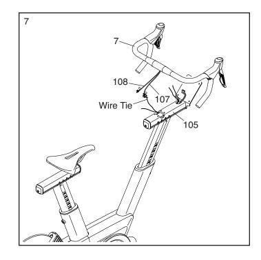
8. **Tip: Avoid pinching the wires.** Hold the Handlebar (7) on the Handlebar Carriage (105), and rotate the Handlebar to the desired angle; **make sure that the Handlebar is centered on the Handlebar Carriage.**
