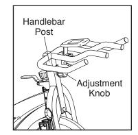
Make sure that the adjustment knob is engaged in an adjustment hole.
