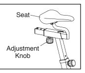
hole in the seat carriage, and firmly tighten the adjustment knob. Make sure that the adjustment knob is engaged in an adjustment hole.
