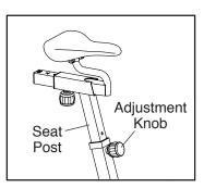
the adjustment knob. Make sure that the adjustment knob is engaged in an adjustment hole.
