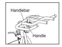
Note: The handle functions like a ratchet. To loosen the handle, turn the handle counterclockwise, pull the handle outward, turn the handle clockwise, push the handle inward, and then turn the handle counterclockwise again. Reverse this process to tighten the handle.
