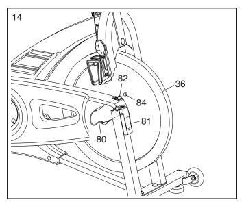
15. After the exercise bike is assembled, inspect it to make sure that it is assembled correctly and that it functions properly. Make sure that all parts are properly tightened before you use the exercise bike. Note: Extra parts may be included. Place a mat beneath the exercise bike to protect the floor.
