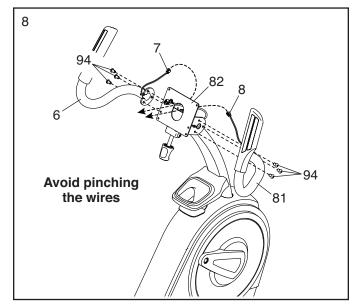
9. While a second person holds the Console (5) near the Console Bracket (82), connect the wires on the Console to the Main Wire (41) and to the Left and Right Pulse Wires (7, 8).
