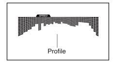
ing segment of the profile represents the current segment of the workout. The height of the flashing segment indicates the target speed for the current segment.
