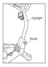
the knob. Move the upright up and down slightly until the pin on the knob snaps into one of the holes in the upright. Then, turn the knob clockwise until it is tight.
