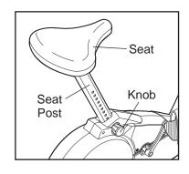
indicated knob counterclockwise two or three turns to loosen it (if the knob is not loosened enough, it may scratch the seat post). Next, pull the knob, slide the seat post to the desired height, and then release the knob. Move the seat post up and down slightly until the pin on the knob snaps into one of the holes in the seat post. Then, turn the knob clockwise until it is tight.
