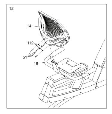
Attach the Seat (12) to the Seat Handlebar (18) with four M6 x 20mm Screws (67) and four M6 Washers (112) (only two of each are shown); start all the Screws, and then tighten them.
