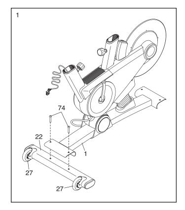
2. Attach the Rear Stabilizer (23) to the Base (1) with two 3/8" x 2 1/4" Patch Screws (74).
