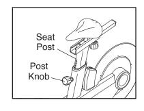
the seat post, and firmly tighten the post knob. Make sure that the post knob is engaged in an adjustment hole.
