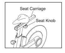
in the seat carriage, and firmly tighten the seat knob. Make sure that the seat knob is engaged in an adjustment hole.
