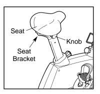
the indicated knob counterclockwise to loosen it, slide the seat carriage forward or backward, and then retighten the knob.
