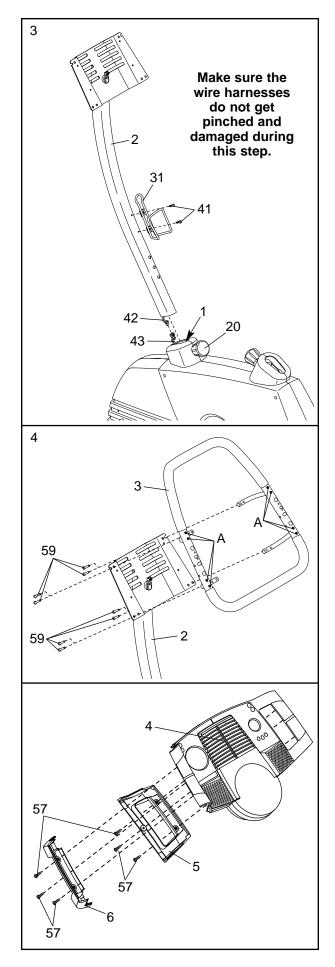
6. While another person holds the Console (4) in the position shown, connect the wire harness on the Console to the Upper Wire Harness (42). Insert the excess wire harness down into the Upright (2).
