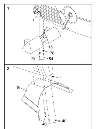
While another person lifts the rear of the Frame (1), attach the Rear Stabilizer (16) to the Frame with four M8 x 33mm Button Screws (40). 3. While another person holds the Upright (2) in the position shown, connect the Upper Wire Harness (42) to the Lower Wire Harness (43). Gently pull the upper end of the Upper Wire Harness to remove any slack from the Wire Harnesses.
