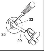
(33). Lightly tap the screwdriver with a hammer to turn the Slotted Bearing Nut counterclockwise until the arms are no longer loose. **Do not overtighten the Slotted Bearing Nut.** When the Slotted Bearing Nut is properly tightened, tighten the Crank Nut.
