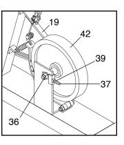
tighten the M8 Flanged Hex Nuts (36). Reattach the side shields.
