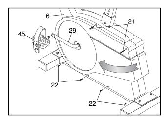
Remove all Screws (21, 22) from the Left Side Shield (6). Grasp both Side Shields at the top and gently pull them apart. Make sure that the arm of the Crank (29) is in the position shown in the drawing above. Hold the Left Side Shield at the rear and pull it gently away from the frame. Work the Left Side Shield forward off the arm of the Crank and remove it.
