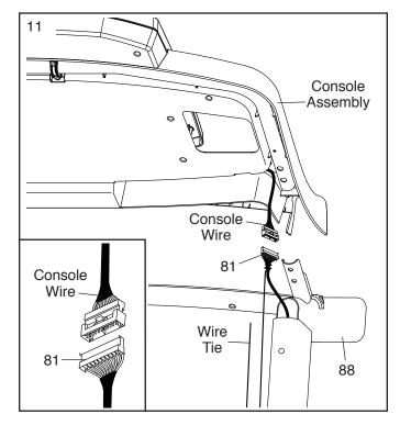
Set the console assembly on the Left Handrail (88) and the Right Handrail (87). Be careful not to pinch any wires. Insert the excess Upright Wire (not shown) into the Left Handrail.
