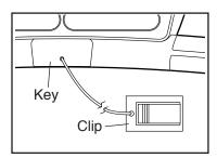
sole. Note: It may take a minute for the console to be ready for use. IMPORTANT: In an emergency, the key can be pulled from the console, causing the walking belt to slow to a stop. Test the clip by carefully taking a few steps backward; if the key is not pulled from the console, adjust the position of the clip.
