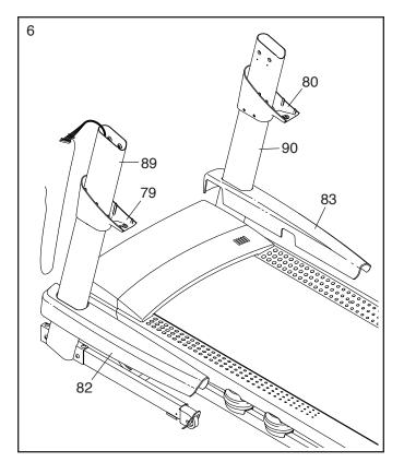
Cut the plastic ties in the Left Handrail (88) and the Right Handrail (not shown). If necessary, press the 5/16" Cage Nuts (31) back into place.
