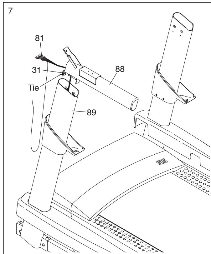
8. Attach the Left Handrail (88) to the Left Upright (89) with two 5/16" x 1" Screws (5), two 5/16" Star Washers (11), and a 5/16" x 1 1/4" Bolt (4). **Do not tighten the Screws and the Bolt yet.**
