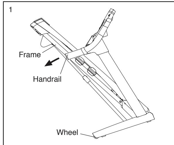
2. Pull back on the handrail until the treadmill will roll on the wheels, and carefully move it to the desired location. **CAUTION: Do not move the treadmill without tipping it back, do not pull on the frame, and do not move the treadmill over an uneven surface.**
