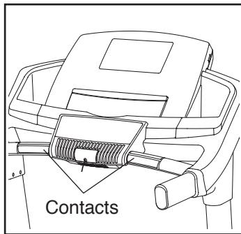
To measure your heart rate, **stand on the foot rails** and hold the contacts with your palms for approximately ten seconds; **avoid moving your hands**. When your pulse is detected, your heart rate will be shown. **For the most accurate heart rate reading, continue to hold the contacts for about 15 seconds.**
