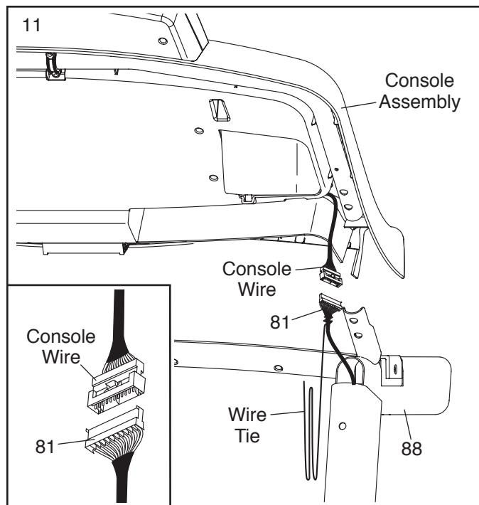
12. Set the console assembly on the Right Handrail (87) and the Left Handrail (88). **Be careful not to pinch any wires.** Insert the excess Upright Wire (not shown) into the Left Handrail.
