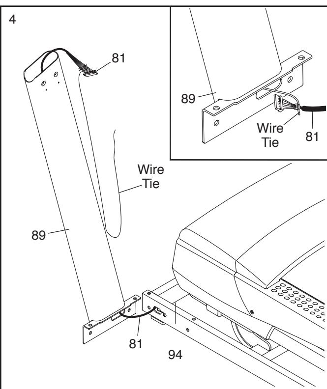
5. Hold the Left Upright (89) against the Base (94). **Be careful not to pinch the Upright Wire (81).** Insert two 3/8" x 1 1/4" Screws (8) with two 3/8" Star Washers (13) and two 3/8" x 2 3/4" Screws (7) into the Left Upright.
