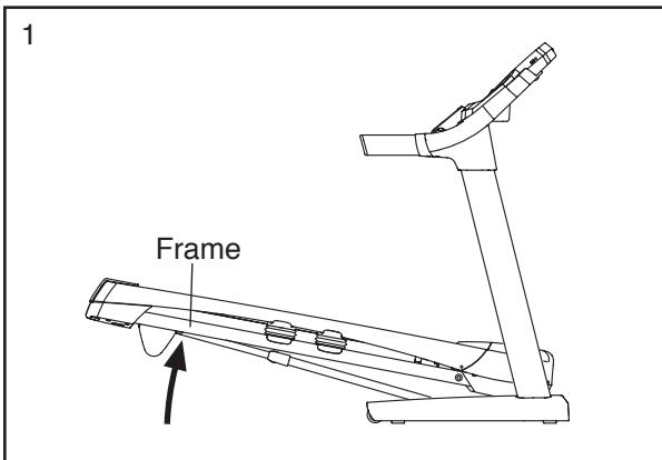
2. Raise the frame until the latch knob locks in the storage position. **CAUTION: Make sure that the latch knob locks.**
