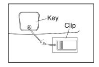
It may take a minute for the console to be ready for use. IMPORTANT: In an emergency, the key can be pulled from the console, causing the walking belt to slow to a stop. Test the clip by carefully taking a few steps backward; if the key is not pulled from the console, adjust the position of the clip.
