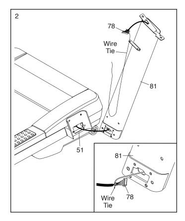
Hold the Right Upright (81) against the Frame (51). Be careful not to pinch the wires. Start a 3/8" x 4 1/4" Screw (2) with a 3/8" Star Washer (9) into the Right Upright and into the Frame; do not fully tighten the Screw yet.
