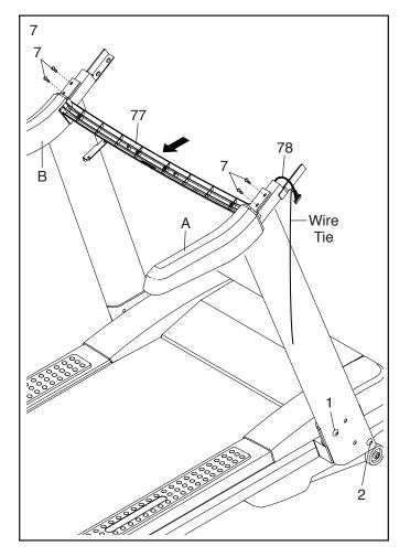
8. With the help of a second person, hold the console assembly near the Right Upright (81) and the Left Upright (not shown). Insert the Upright Wire (78) through the looped plastic ties on the bottom of the console assembly.
