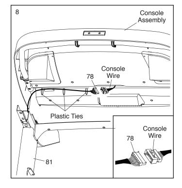
9. Route the Upright Wire (78) as shown so that it does not get pinched as you set the console assembly onto the right handrail assembly (B) and the left handrail assembly (not shown).
