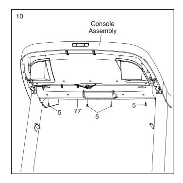
Attach the console assembly with four 5/16" x 3/4" Screws (105), four 5/16" Flat Washers (103), and four 3/8" External Star Washers (104) as shown. Start all four Screws, and then tighten them.
