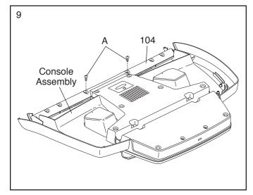
10. IMPORTANT: To avoid damaging the Crossbar (104), do not use power tools and do not overtighten the #10 x 3/4" Screws (2).
