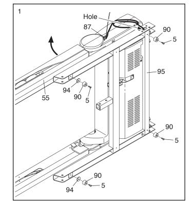
2. **See the inset drawing.** Cut the plastic tie near the Upright Wire (87).
