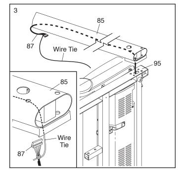
4. Hold the Right Upright (85) against the Base (95). Be careful not to pinch the Upright Wire (87). Insert two 3/8" x 4" Screws (7) with two 3/8" Star Washers (11) and a 3/8" x 1 1/2" Screw (14) with a 3/8" Star Washer (11) into the Right Upright.
