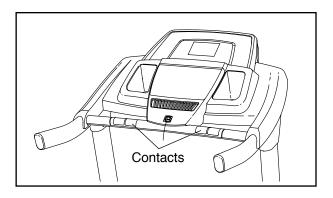
To measure your heart rate, stand on the foot rails and hold the pulse bar with your palms on the metal contacts for approximately ten seconds; avoid moving your hands. When your pulse is detected, a heart symbol in the calorie display will flash each time your heart beats, one or two dashes will appear, and then your heart rate will be shown. For the most accurate heart rate reading, continue to hold the contacts for about 15 seconds.
