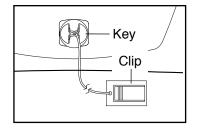
the console. After a moment, the displays will light. IMPORTANT: In an emergency, the key can be pulled from the console, causing the walking belt to slow to a stop. Test the clip by carefully taking a few steps backward; if the key is not pulled from the console, adjust the position of the clip.
