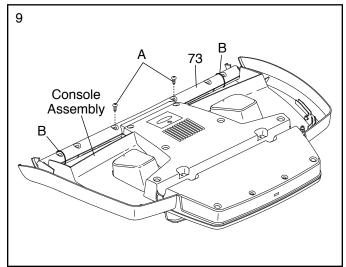
10. IMPORTANT: To avoid damaging the Crossbar (73), do not use power tools and do not overtighten the #10 x 3/4" Screws (2).
