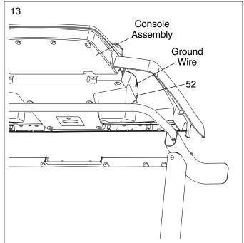
14. Set the console assembly on the Left and Right Handrails (82, 83). **Be careful not to pinch any wires.** Insert the excess Upright Wire (87) into the Right Handrail.
