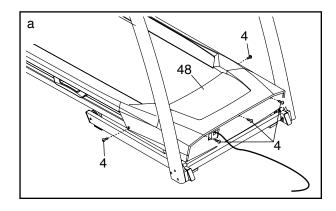
Carefully lift the Motor Hood (48) upward, and then slide it forward and off. Make sure that the Motor Hood does not get caught by the tabs on the sides of the Motor Hood.
