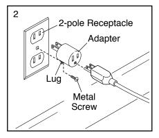
The lug or wire extending from the adapter must be connected with a metal screw to a permanent ground such as a properly grounded outlet box cover. Some 2-pole receptacle outlet box covers are not grounded. Before using an adapter, contact a qualified electrician to determine whether the outlet box cover is grounded. The temporary adapter should be used only until a properly grounded outlet can be installed by a qualified electrician.
