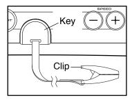
light. IMPORTANT: In an emergency, the key can be pulled from the console, causing the walking belt to slow to a stop. Test the clip by carefully taking a few steps backward; if the key is not pulled from the console, adjust the position of the clip.
