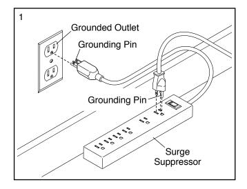
A temporary adapter may be used to connect the surge suppressor to a 2-pole receptacle if a properly grounded outlet is not available.
