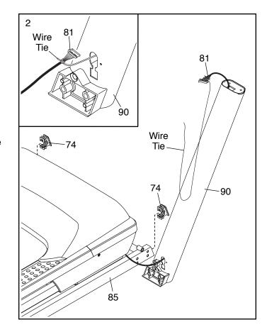
3. Lay the Right Upright (90) near the Base (85). Press the Grommet (77) into the square hole in the Right Upright. Make sure not to pinch the ground wire.
