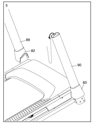
6. Set a Handrail (84) onto the Right Upright (90). Make sure that the Upright Wire (81) is not pinched.
