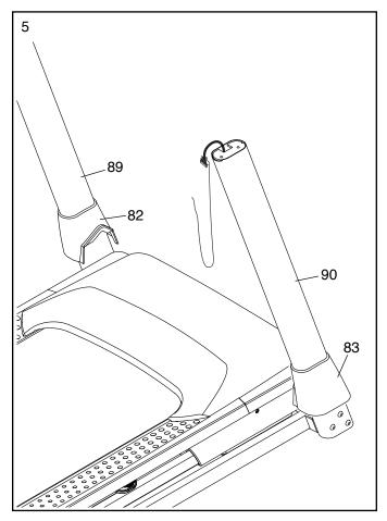
Set a Handrail (84) onto the Right Upright (90). Make sure that the Upright Wire (81) is not pinched.
